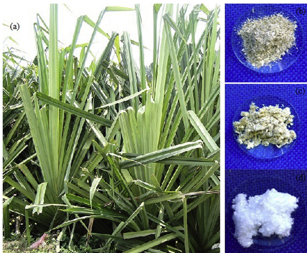
Fig. 1. Photographs of (a) the mengkuang plant, (b) raw ground leaves, (c) alkali-treated leaves, and (d) bleached leaves.
